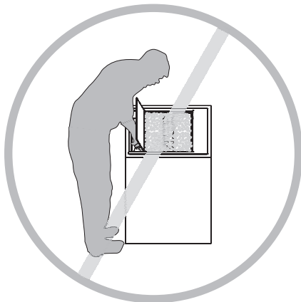
NEVER LEAN OVER FIREPIT WHEN LIGHTING BURNER
