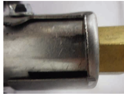
Figure 1 - Air shutter at 1/8-inch opening
